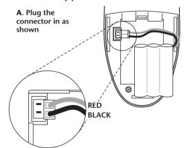
B. Tuck the wires in and lay the battery pack in the compartment
