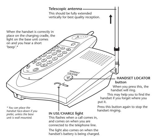
IMPORTANT — before using the handset for the first time, you need to leave it on the base unit for 12 hours so that the battery becomes fully charged.
